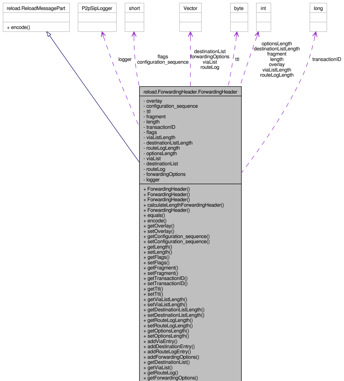
Figure 3.2: Class diagram of the Forwarding Header
